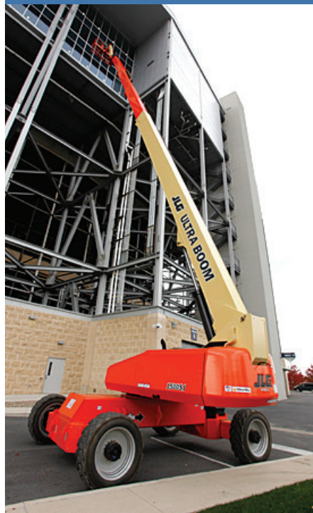
The JLG 1350SJP Ultra Series Telescopic Boom Lift is equipped with a fuel-efficient Tier 4 engine and can go from ground to 135 ft up in 95 seconds.
